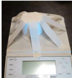
If you do not have the original packaging you may want to protect the pin with a plastic cap or cut a ring out of a paper roll and tape it in place as shown. This will keep anything from hitting the pin and damaging the cell.
